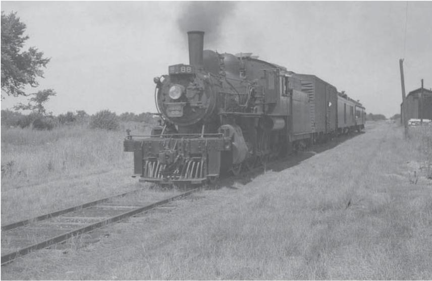
*It's July 25, 1953 and CNR 2-6-0 #88 arrives at Port Rowan with the mixed train in tow. The train is on the main. To the right, barely visible in the grass, is the team track. The runaround track is to the left – similarly overgrown. The barn at right blocks the view of the elevated coal track. (Elmer Treloar photo, Keith Sirman Collection – used with permission)*
