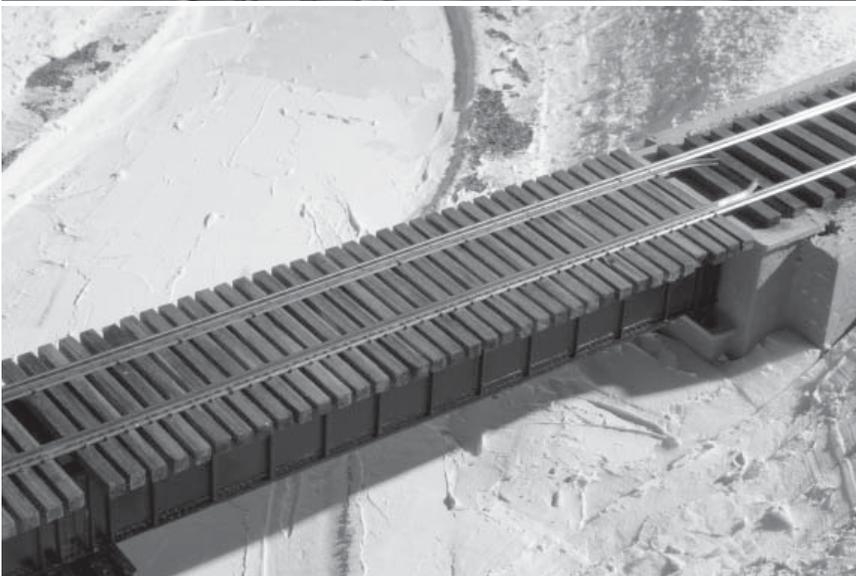
(Bottom left) Undertaking a relatively simple layout such as this allows the author to invest more time detailing his scenes. A case in point is this bridge, on which the running rails are spiked every tie. The guardrails are spiked every fourth tie or so. The bridge will receive more detail and weathering before it's installed permanently.
